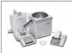
LV11 automatic feeder for automatic loading of small items on the balance
