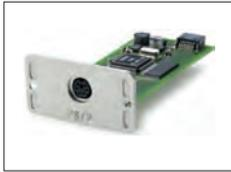
PS/2 option: Interface for connecting commercial keyboards and barcode readers
