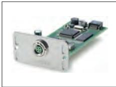
LocalCAN option: Interface for connection of up to 5 LC (LocalCAN) instruments
